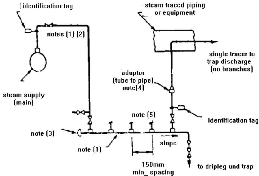
**TYPICAL ARRANGEMENT OF PIPING AND TUBING COMPONENTS FOR STEAM SUPPLY AND DISTRIBUTION**
